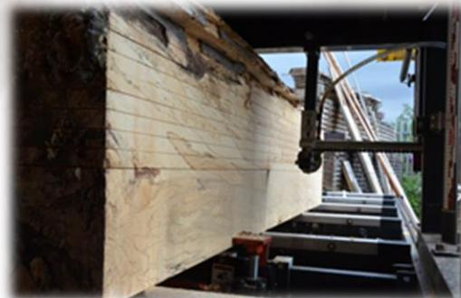
Once in our yard where it is milled on the Timberking 2200, the UK's largest narrow gauge mill (capable of 6.5m length, 840mm in width and 735mm high).
